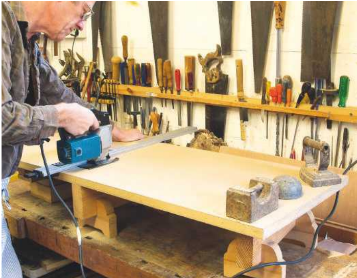
▲ Pic.2 Cutting the MDF base: Michael's not keen on MDF but it does the job – for an easy planing technique follow Pics.3-6 over page
